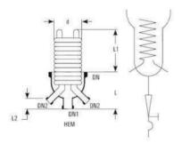
Product coolers are used for cooling of liquids, typically, for the cooling of distillates from the distillation columns.
